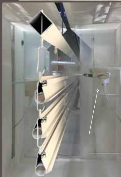
Our 31,000 square foot powder coating facility is fully automated from start to finish. Because of our 313-foot continuous powder coat line, we have the capability to coat frame parts and extrusions up to 30 feet in length at a line speed of 7 feet per minute.
